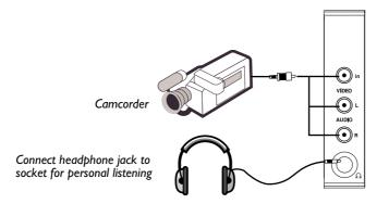
For more convenient direct playback connections, the Side Audio/Video Input sockets allow for quick and easy connections, particularly Camcorder tape recordings.
